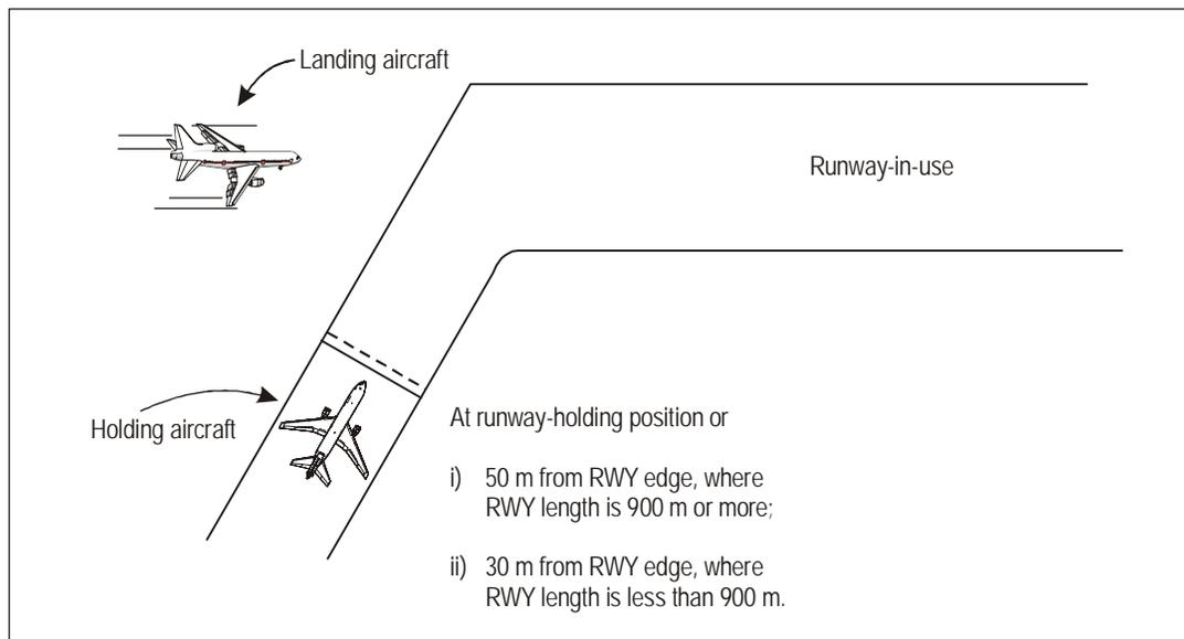
**Figure 7-2. Method of holding aircraft (see 7.6.3.1.3.2)**
