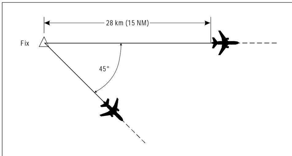
Figure 5-4. Separation using dead reckoning (see 5.4.1.2.1.2 c))
