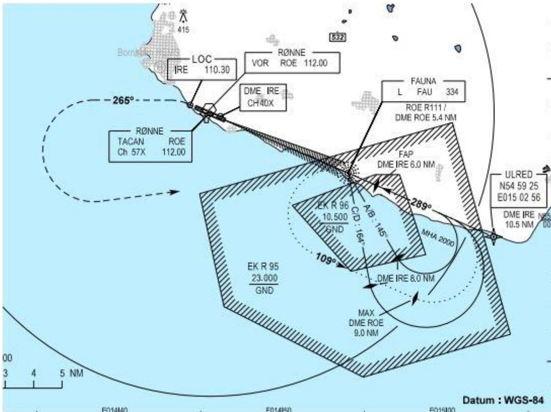
When an aircraft is inbound FAU, they will after the WP turn "downwind/base". Be noted the turning curve is different based of aircraft type. After the "Teardrop turn" they will establish on ILS.
